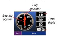
When you are navigating a route, the compass rotates and the bug indicator shows the direction you should be travelling to stay on the route. The bearing pointer indicates your current direction. If the arrow points up, you are going directly to the destination. If the arrow points any other direction, navigate the direction of the bug indicator until the arrow points up.
